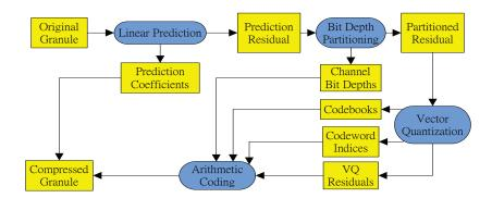
Fig. 2. The data flow diagram for PPVQ.
